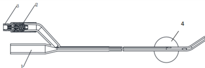
1 drainage funnel 2 Inflation Funnel 3 Valve 4 Balloon
